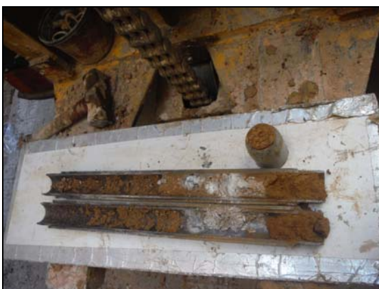
Foto 11: Sondage S-3, SPT a 4,2 metres
