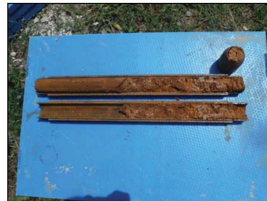
Foto 16: Sondeig S-2, SPT a 6,0 metres.
